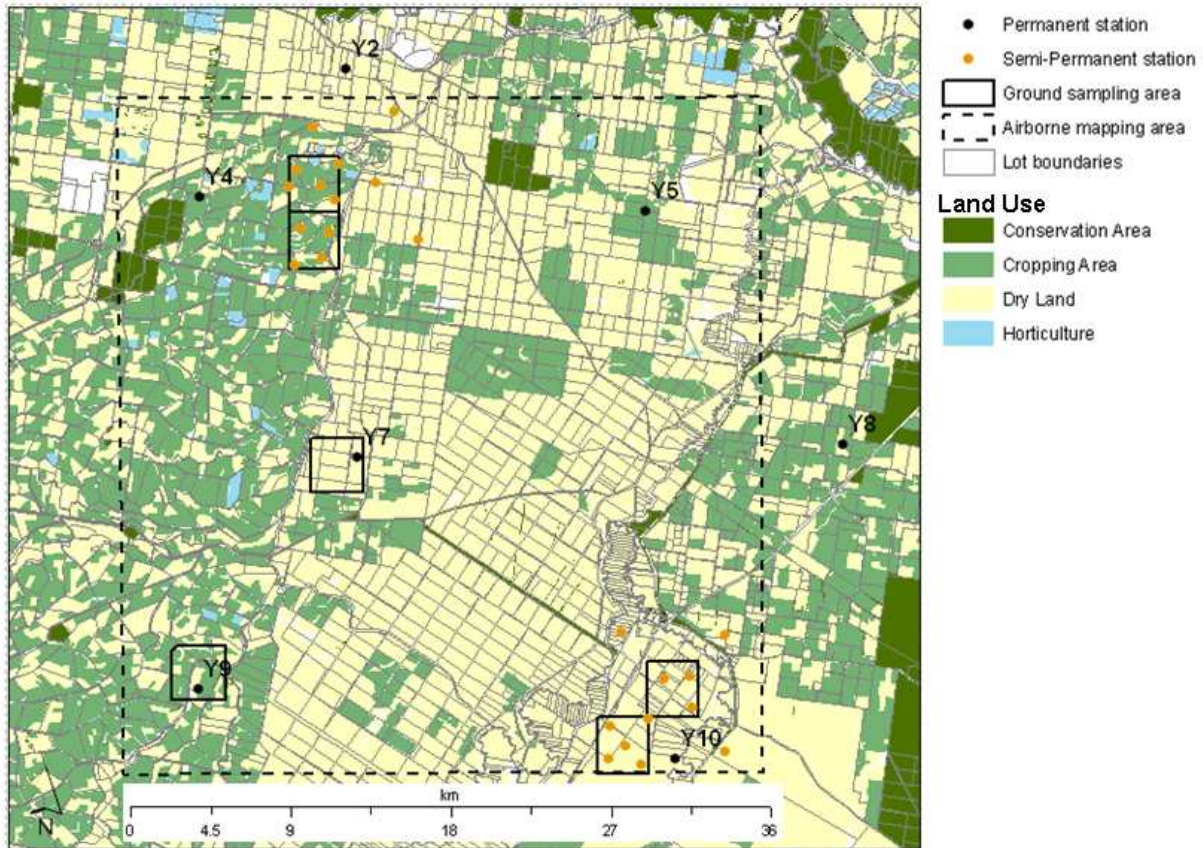
Figure 4-3. The Yanco site is a 60km box with approximately one third of irrigated area (Coleambally Irrigation Area). The six ground sampling areas of SMAPEX and the soil moisture monitoring networks are indicated.
