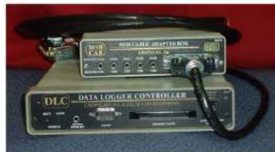
Figure D- 2. Data logger controller &amp; cable adapter box
