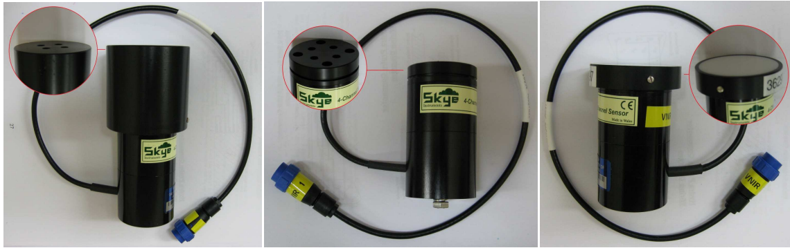
Figure 3-7. Multi-spectral sensors; downward looking sensors (left and middle) and upward looking sensor with cosine diffuser fitted (right).
