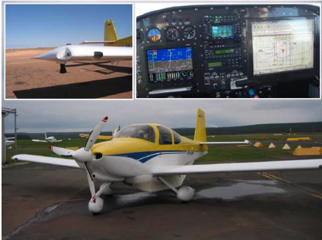
Figure 3-1. Experimental ESV aircraft showing a wingtip installation in the left inset, and the cockpit with cockpit computer display in the right inset.
