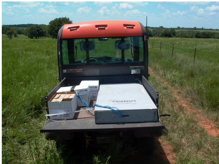
Figure 3-10. The COSMOS rover during a transect in Tucson, Arizona, USA.
