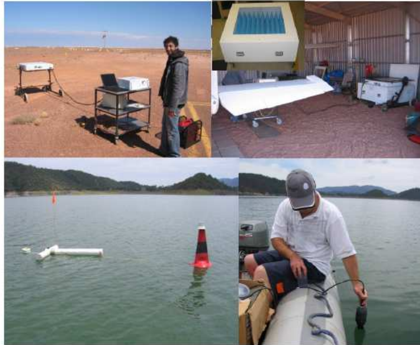
Figure 5-6. Upper left: undertaking a sky cold point calibration with PLMR; upper right: undertaking a warm point calibration with the calibration box shown in the inset; lower left: the buoy used to monitor water temperature and salinity; lower right: undertaking a boat transect of water salinity and temperature.
