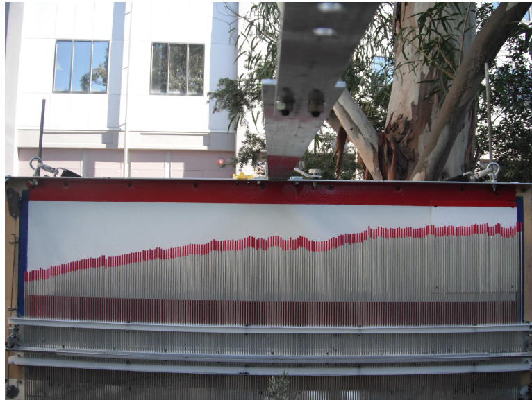
Figure 7-5. Pin profiler for surface roughness measurements.
